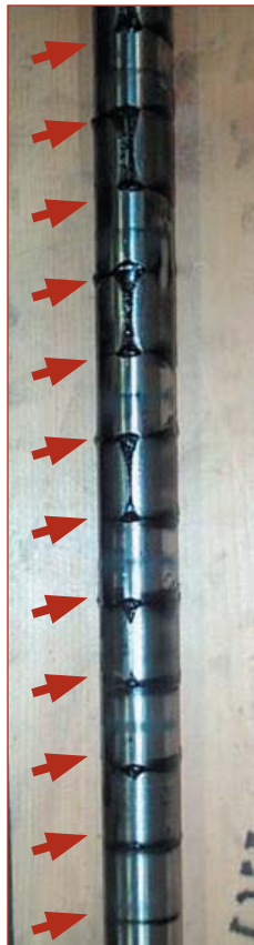
upper left: Kinecor's hydraulic test bench lower left & right: FilterMaster magnetic rod with trapped ferrous contamination (indicated by arrows)
