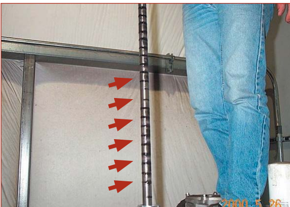
upper left: Kinecor's hydraulic test bench lower left & right: FilterMaster magnetic rod with trapped ferrous contamination (indicated by arrows)
